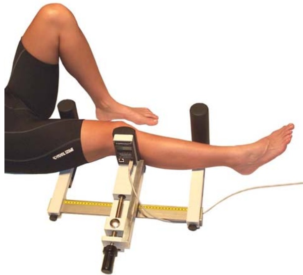
Figure 4.8.2 – Right Knee mounted in stress device for MCL exam
