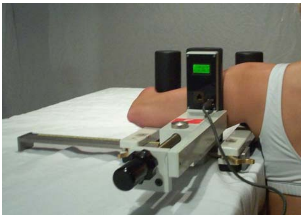
Figure 4.11.2 – Left Shoulder mounted in stress device for anterior exam with no rotation
